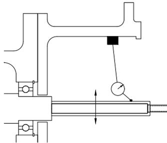
Figure 3: Bearing Fit
