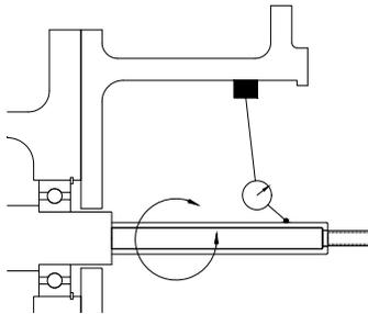
Figure 2: Shaft Runout
